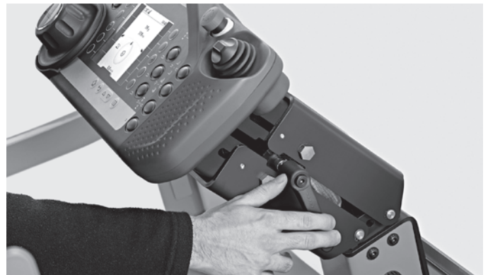
Three-dimensional positioning of the control panel
