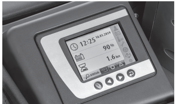
The colour display with language-independent symbols shows all of the important functions at a glance
