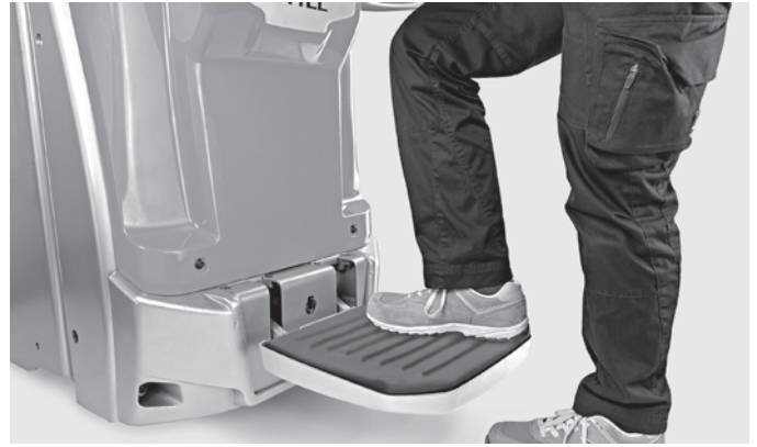
Adjustable side arms and air-sprung stand-on platform adjustable to individual driver weight
