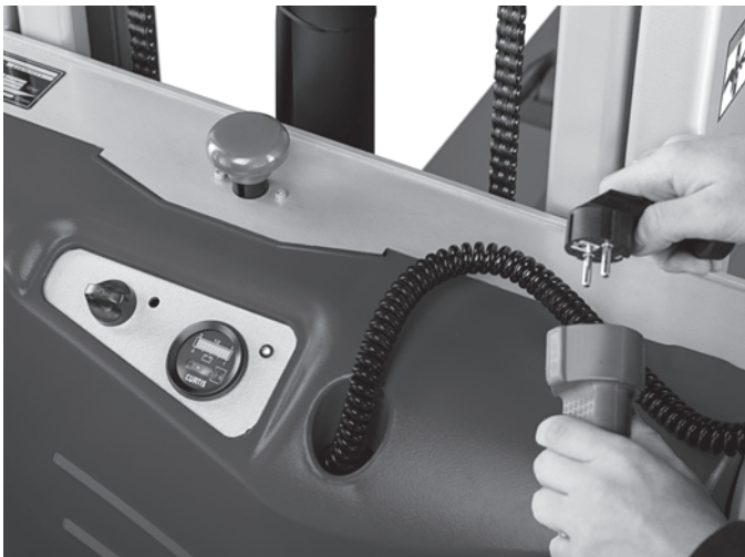
Built-in charger guarantees maximum availability and enables decentralised charging
