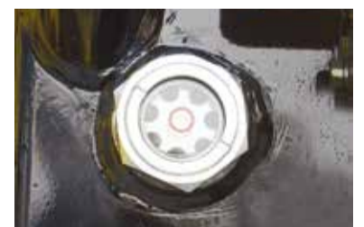
Hydraulic oil level gauge
