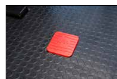
New floor mat & Dead man switch
