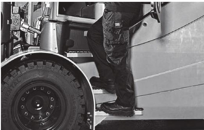
Non-slip steps visible from the top for safe access and exit
